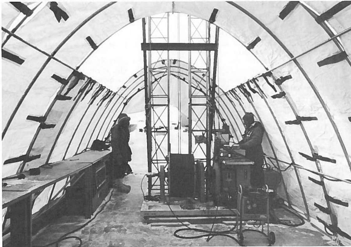
Figure 1. Winch platform including winch drum, tower assembly and control panel inside the canvas-covered drill shelter at the South Pole, December 1982.
