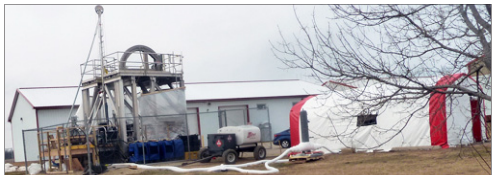
(Left) The 10-inch (0.25 meter) ice column being formed in the casing insert. (Right) The ASIG Drill test site at the UW PSL. At left, the ASIG Drill rig sits on a wooden deck with hydraulic engines in blue covers and wire-line tower visible above pre-existing aluminum platform; at center, a 500 gallon (1890 L) diesel wagon; at right, the drill tent housing the chiller; frosted glycol supply hoses visible in foreground. Credit: Chris Gibson
